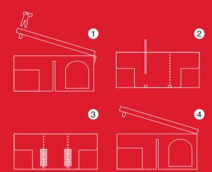
Insert the key provided into one set of fastening holes on the lid and turn to release the fastening.
